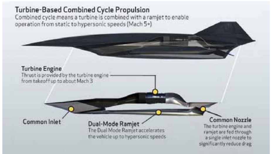
The American Defense Advanced Research Projects Agency (DARPA), as well as the Beijing Power Machinery Research Institute (and probably many more military/aerospace institutions) are working on building “combined cycle” or “full range” engines which incorporate a turbojet along with an integral ramjet/scramjet engine to allow full operation from a standstill to Mach 5+ hypersonic flight.
