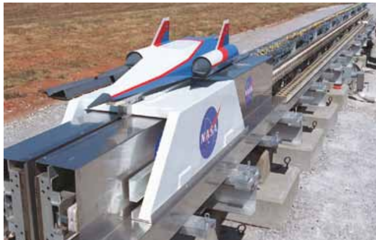
Different technologies to catapult-launch a spacecraft have been tested by NASA, including this magnetic levitation (maglev) system evaluated at NASA's Marshall Space Flight Center.
