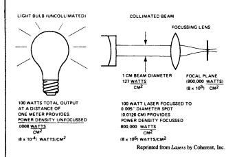
A laser produces radiative light energy in a coherent form: all the light rays are of the same wavelength and are traveling in the same direction. A laser converts incoherent energy, such as white light or electrical energy into light of one specific wavelength, or color.
