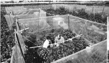
Above: Open-top enclosures of clear polyethylene are used to study the effects atmospheric  $CO_2$  enrichment on the growth and water use of cotton at Phoenix, Arizona. Pure  $CO_2$  gas is mixed with ambient air and continually released into the treatment chambers through perforated tubes which lie upon the ground. In the hot environment of summer, a doubling of the air's  $CO_2$  content practically doubles the yields of the plants.
