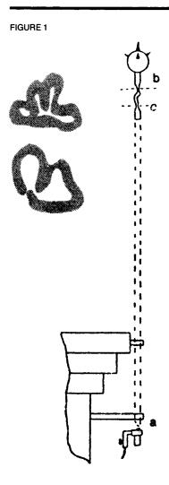
Drawings of the crosssections of the copper lightning rod that was crushed by the passage of a lightning bolt.
