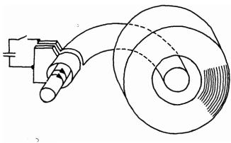
Typical geometrics for pinch-effect apparatus.
