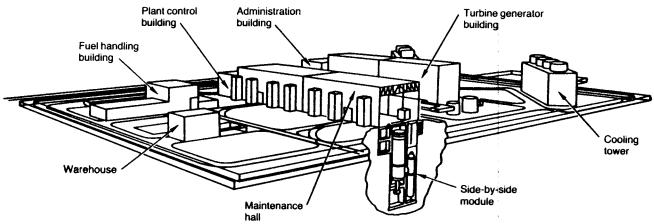
This General Atomics power plant design has four MHTGR modules, each at 135 megawatts-electric, for a total power output of about 540 megawatts. The reactor module, called the nuclear island, is completely separate from the electric power generating system. It is housed in a below-ground concrete silo. Each of the four nuclear islands is an independent confinement structure, with its own exhaust system.
