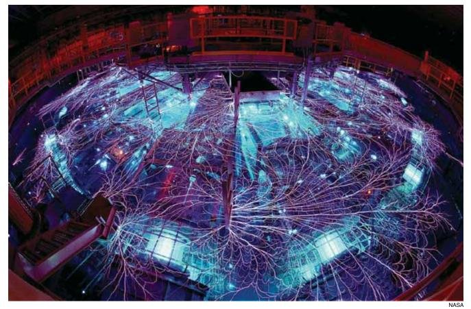
The continued survival of mankind exists depends upon the vigorous advance of an increase in power, as defined by nuclear fission and thermonuclear fusion. Shown: Sandia National Laboratories' "Z Machine," the world's largest X-ray generator, which, it is hoped, will, one day, ignite a nuclear fusion reaction.
