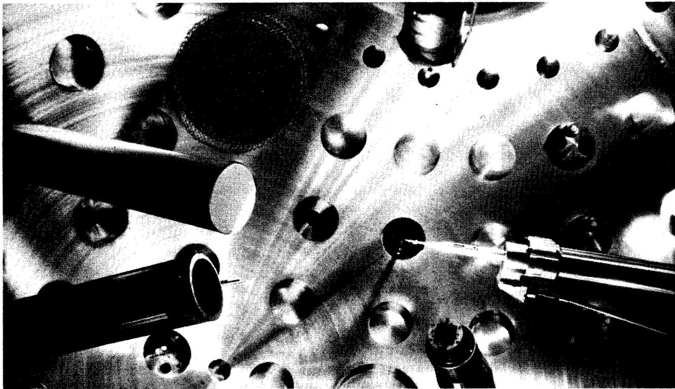
*Inside the target chamber of the Shiva laser fusion apparatus at Lawrence Livermore Laboratory in California: these classified experiments led to the nuclear-pumped x-ray laser. Above, 30 trillion watts of optical power are focused from the top and bottom onto fusion fuel targets at the tip of the positioner at right.*
