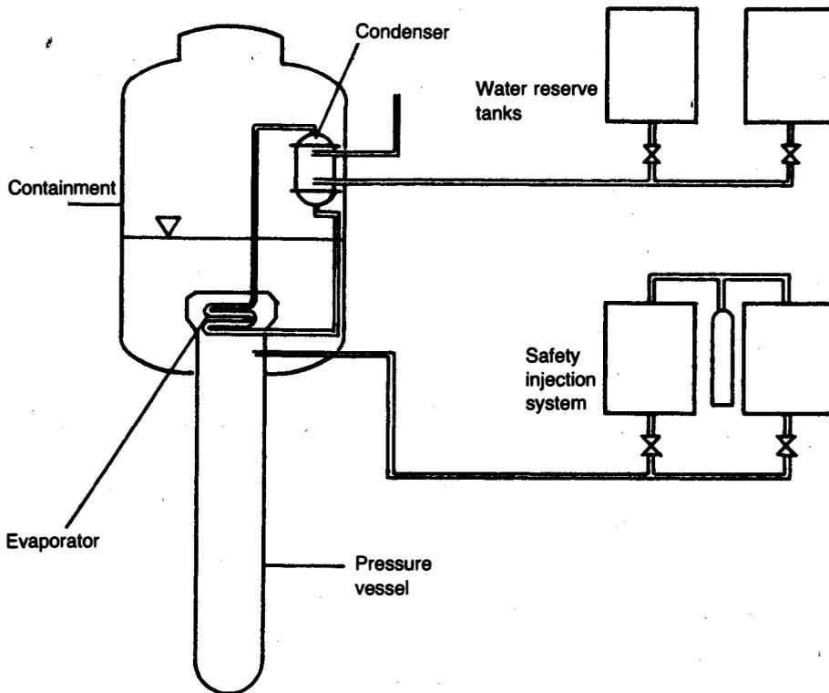
ing power transients, passing them into the surrounding pool as increases in temperature which can be radiated away. There are only very small pressure drops in any of the piping and cooling tubes, and thus the reactor is both safe and highly reliable in operation.
