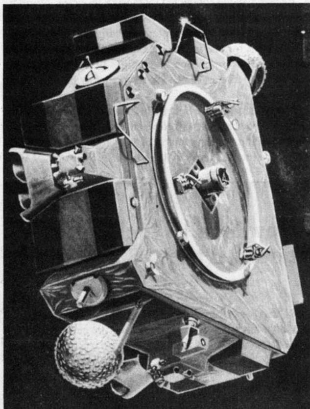
*The Orbital Maneuvering Vehicle is a reusable, free-flying space vehicle designed to enhance the Shuttle orbiter's payload delivery and retrieval capabilities. It can inspect satellites and retrieve them to a space station or the Shuttle orbiter, and can perform a variety of on-orbit tasks.*
