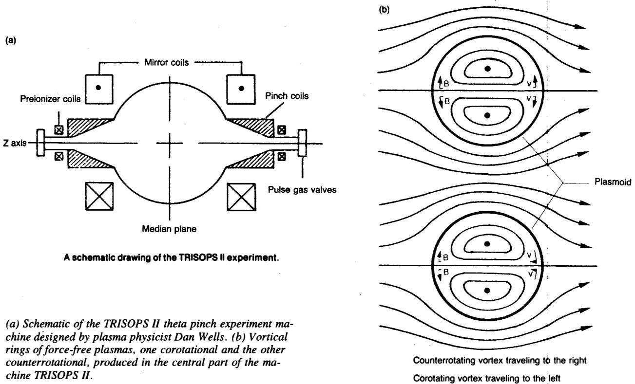
A schematic drawing of the TRISOPS II experiment.
