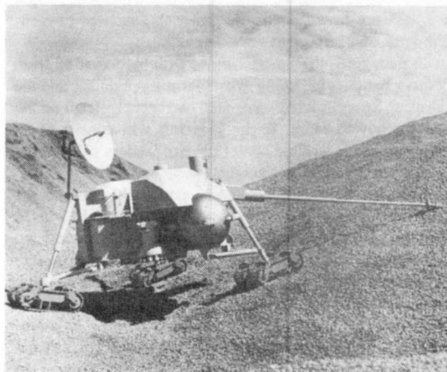
*This scale model of a mobile Mars lander was built and tested by Martin Marietta Aerospace for NASA. The mobile laboratory travels on three loop tracks, and would be able to sample Martian soil, and repeat experiments at various locations on the planet.*
