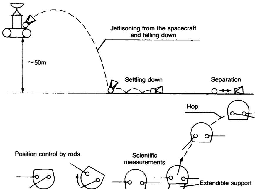
*One of the landers planned for the 1988 Soviet Phobos mission is a hopper, seen here. It will be jettisoned from an orbiting spacecraft, settle down, and then hop from spot to spot to study the soil composition of the tiny moon. It will be able to hop about 20 meters at a time.*
