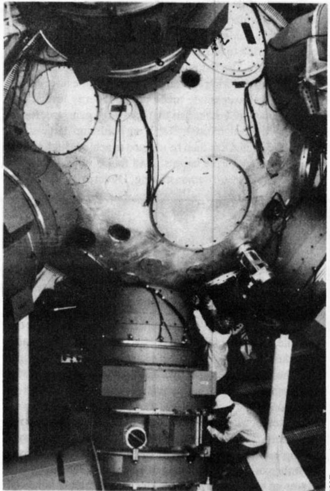
*Laser technicians install diagnostic instruments on the Nova target chamber. Nova, at Lawrence Livermore National Laboratory, is the world's most powerful laser, and is helping scientists to harness fusion energy.*
