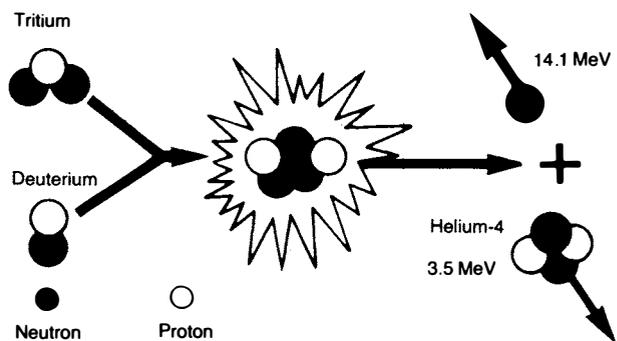
To attain fusion, two nuclei of hydrogen, the basic fusion fuel, must join together. This generates one helium nucleus from every two nuclei of hydrogen and liberates energy in the process.
