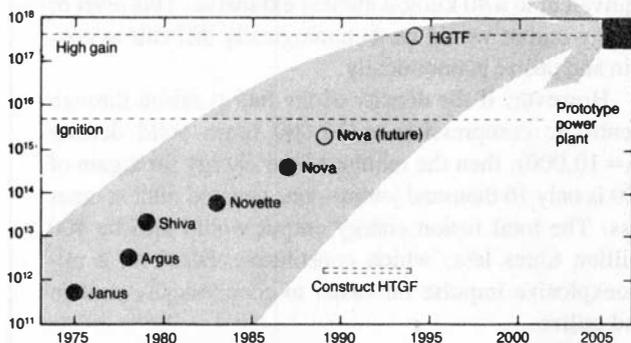
There has been continuous progress in the inertial confinement fusion program, moving toward the conditions required for commercial fusion energy in the early 21st century. This figure shows (vertical axis) the product of temperature, density and confinement times achieved in experiments at Lawrence Livermore National Laboratory since 1975. The temperature, density, confinement time product is given in units of kilovolts, nuclei per cubic centimeter, and seconds, respectively.
