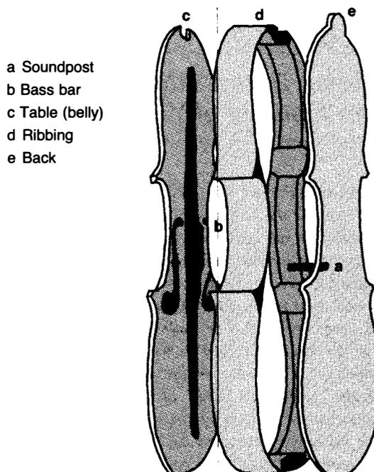
*The soundpost (a) set under the right foot of the bridge, transmits vibrations to the back of the violin (e). The bass bar (b), glued to the back of the table (c), stiffens the body and distributes the vibrations.*
