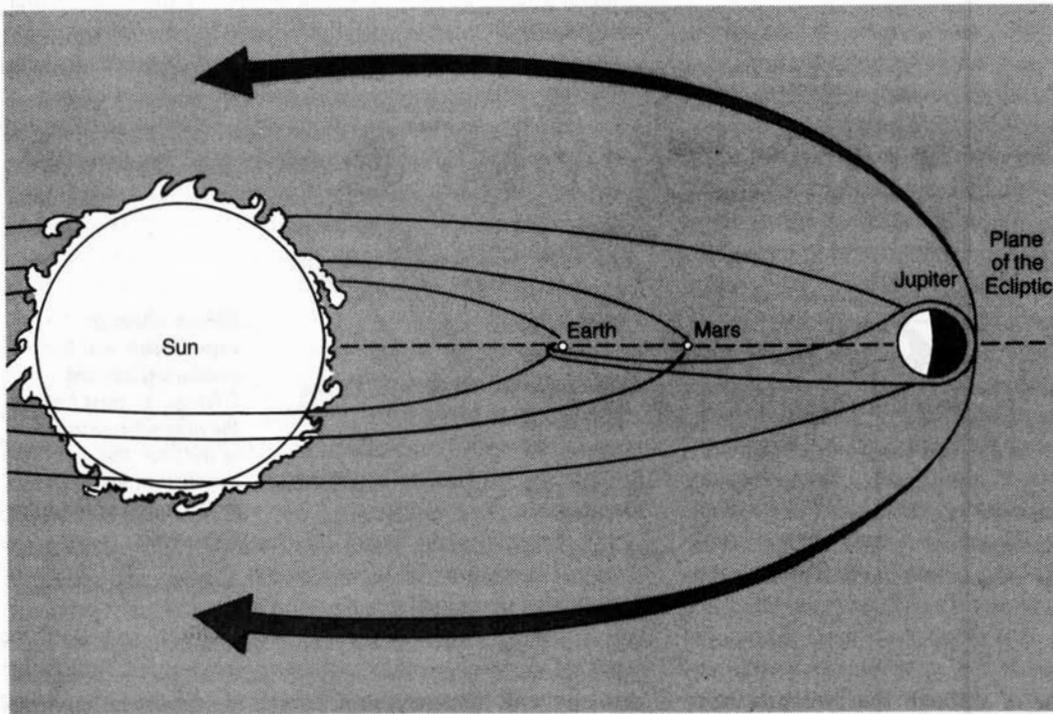
*The two-spacecraft International Solar Polar Mission: According to the original plan, two spacecraft, launched simultaneously from the Shuttle, would have orbited the poles of the Sun at the same time. Thus, a genuine three-dimensional view of the Sun would have been possible.*
