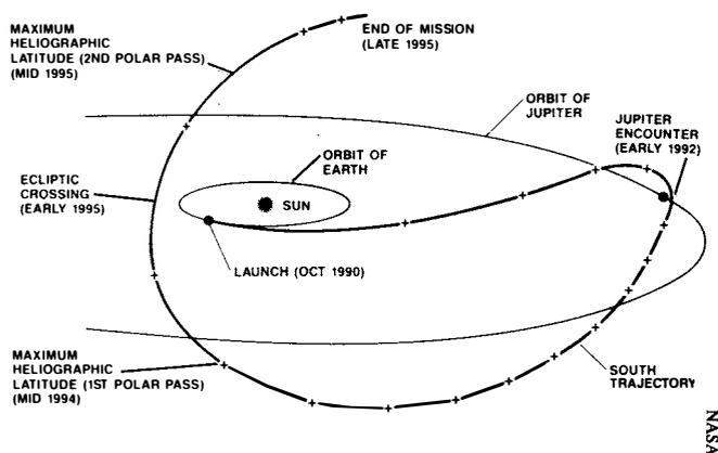
*The Ulysses spacecraft is now on its way to a February 1992 encounter with Jupiter. A Jovian gravity assist will boost it south of the planetary plane of the ecliptic to place it under the Sun's south pole in mid-1994. One year later, it will view the Sun from above its north polar region.*
