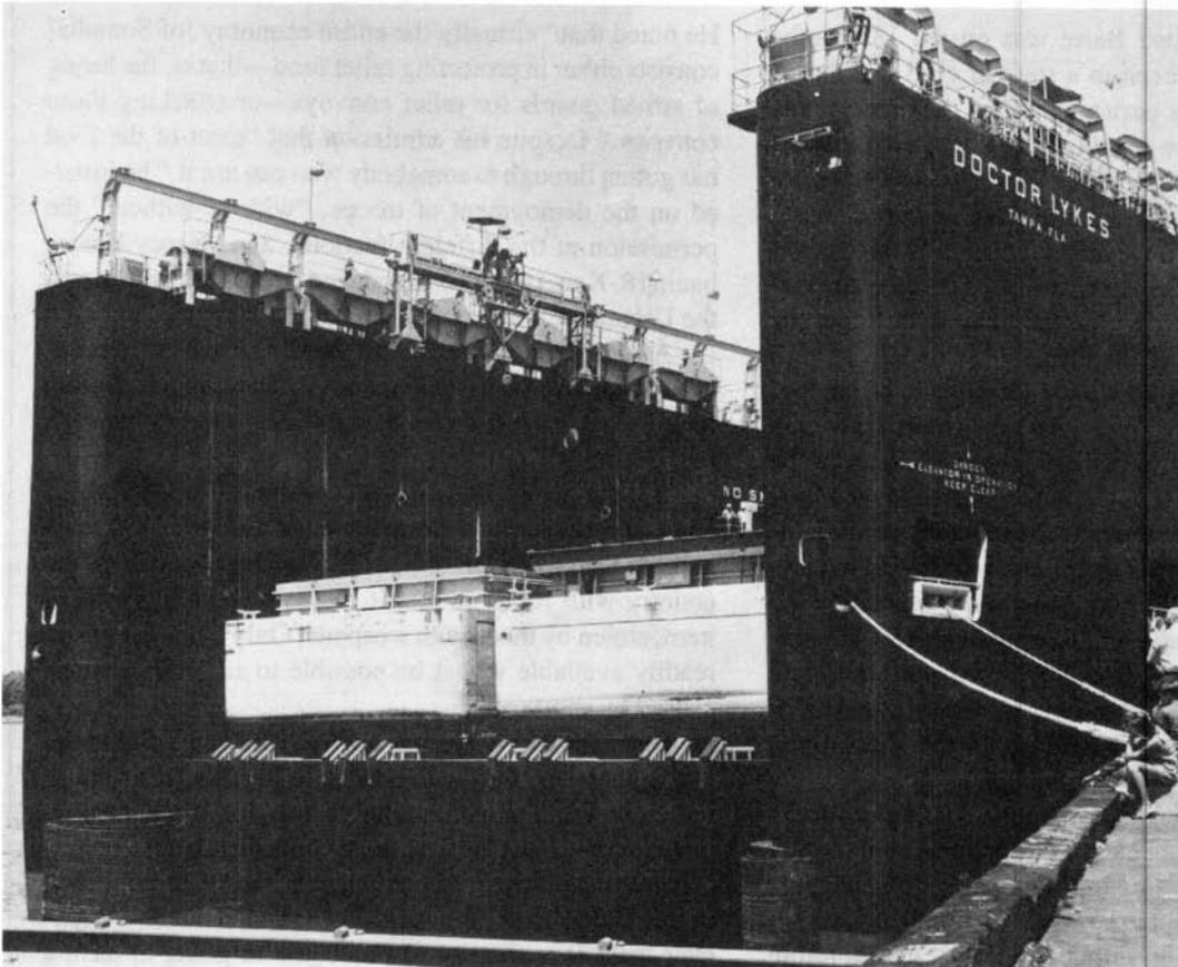
*Loaded barges lower off the stern platform elevator of Doctor Lykes, a Lighter Aboard Ship (LASH) vessel, which carries barges and comes equipped with a self-contained loading and unloading elevator. Cargo containers on the deck are loaded with grain and can become independent at the point of debarkation. Such technologies allow a rapid, effective relief effort.*
