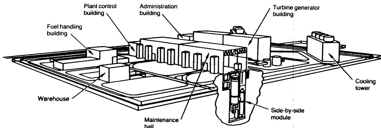
*This General Atomics power plant design has four MHTGR modules, each at 135 megawatts-electric, for a total power output of about 540 megawatts. The reactor module, called the nuclear island, is completely separate from the electric power generating system. It is housed in a below-ground concrete silo. Each of the four nuclear islands is an independent confinement structure, with its own exhaust system.*
