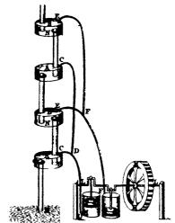
In 1687, Papin illustrated the operation of his pneumatic pump by constructing a model fountain. Water was raised by alternate suction and pressure exerted by a pair of air pumps.
