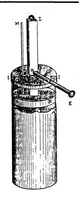
The first steam engine using a piston and cylinder was invented by Papin in 1690. He proposed to use steam instead of gunpowder to create a vacuum under a piston.
