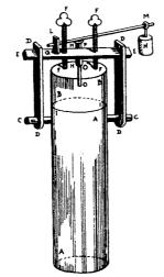
Denis Papin's 1680 steam pressure cooker or "digester," with an adjustable safety valve at the top.
