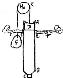
Christiaan Huygens designed this earliest internal combustion engine in 1673, using a charge of gunpowder to create a vacuum in a cylinder under a piston.
