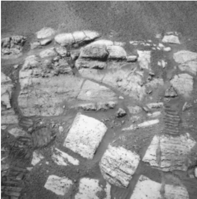
Two of the rocks in the El Capitán formation that Opportunity targeted for detailed study, were the triangular-shaped McKittrick—in the center of this photograph—and Guadalupe, further up. Both have been drilled into with the rover’s Rock Abrasion Tool, indicated by the circular drilling patterns seen in the photo.
