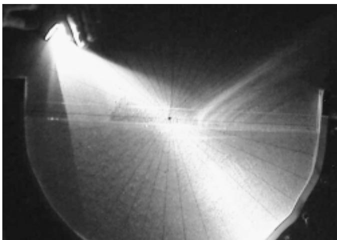
*In an experiment conducted by the LYM, the path of light is seen to change direction when it passes from air to water.*
