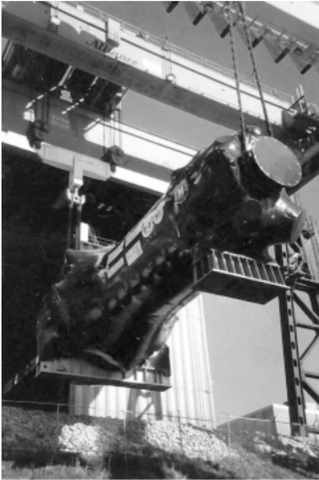
A nuclear power plant steam generator is lifted with overhead cranes from the shop floor onto a barge for shipment.
