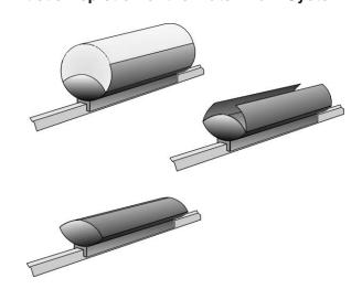
Each Water Train vehicle has a bladder that holds 50,000 gallons of water. Thus a 200-vehicle unit train could deliver 10 million gallons per trip. A Water Train vehicle with bladder filled is shown at top. For the return trip, the bladders would be collapsed (bottom), in order to reduce air drag.
