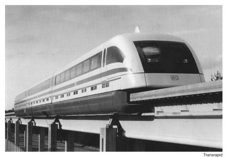
In the German Transrapid system, electromagnets are attracted upwards to iron rails at the edges of a T-shaped guideway beam, providing the magnetic force to levitate the vehicle.
