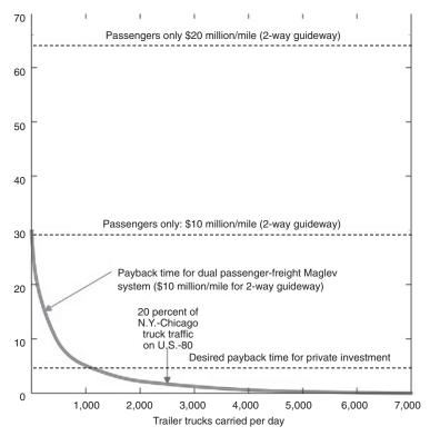
The figure shows the time it takes to pay back the cost of the Maglev guideway carrying passengers only, and a dual system that carries both passengers and freight. The conditions used in the calculation are 3 million passengers per year, at 10 cents per passenger mile, net revenue, and 25 tons per trailer truck at 20 cents per ton-mile revenue.
