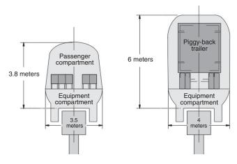
The schematic drawings show the relative size and configuration of Maglev-2000 passenger and freight vehicles.
