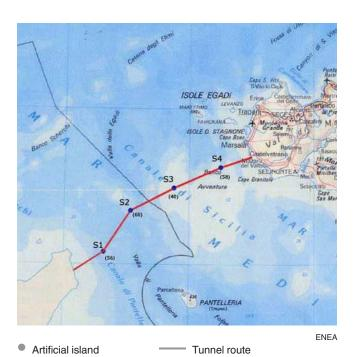
Planimetric scheme for the tunnel under the Channel of Sicily for the Europe-Africa rail link.
