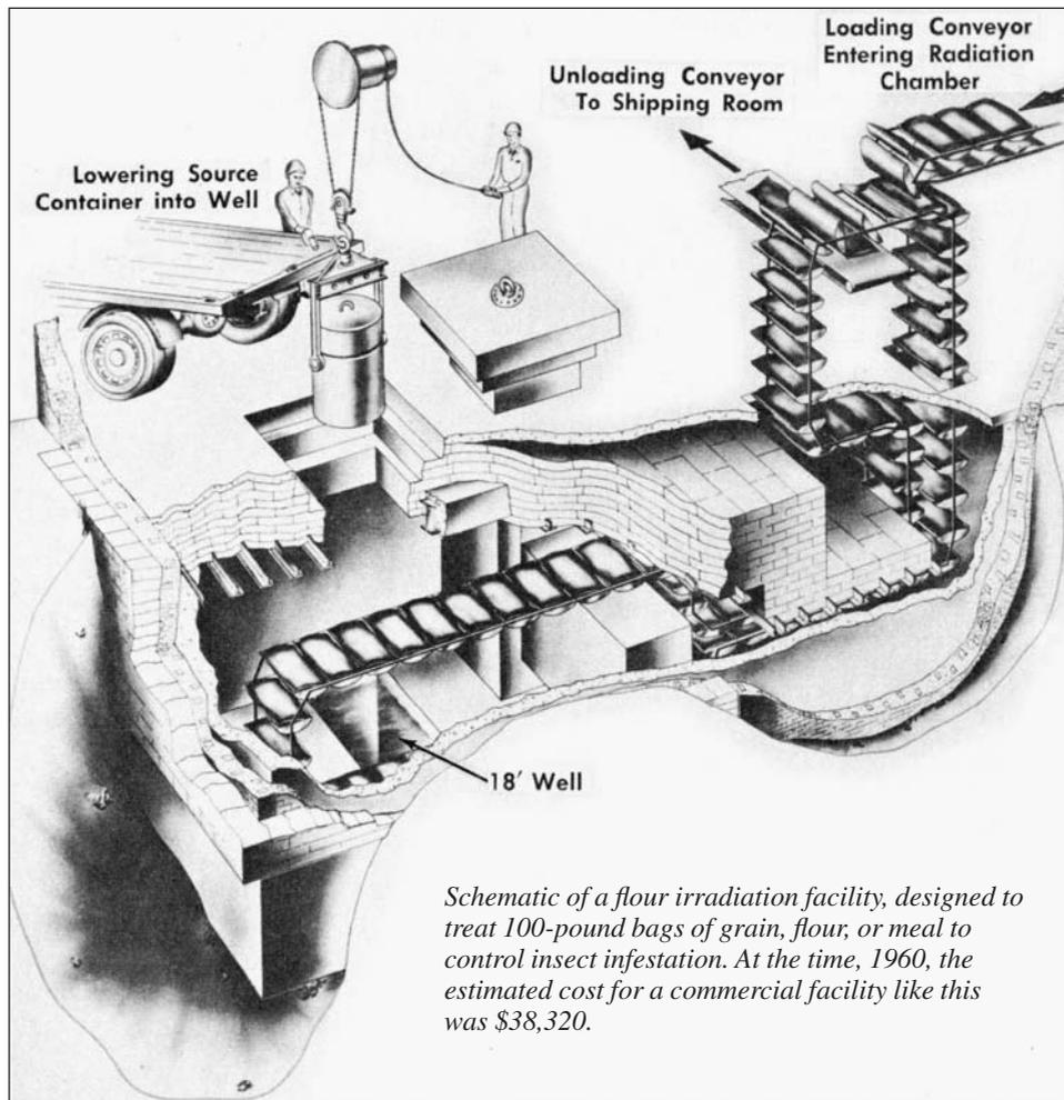
*Schematic of a flour irradiation facility, designed to treat 100-pound bags of grain, flour, or meal to control insect infestation. At the time, 1960, the estimated cost for a commercial facility like this was \$38,320.*
