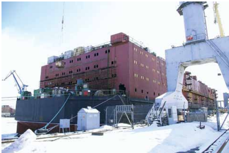
To supply the region with energy, the Russian government has decided to place eight floating nuclear power plants along the northern coast. This photo shows the Akademik Lomonosov, a floating nuclear power station, being launched at Baltiyskiy shipyard in St. Petersburg.
