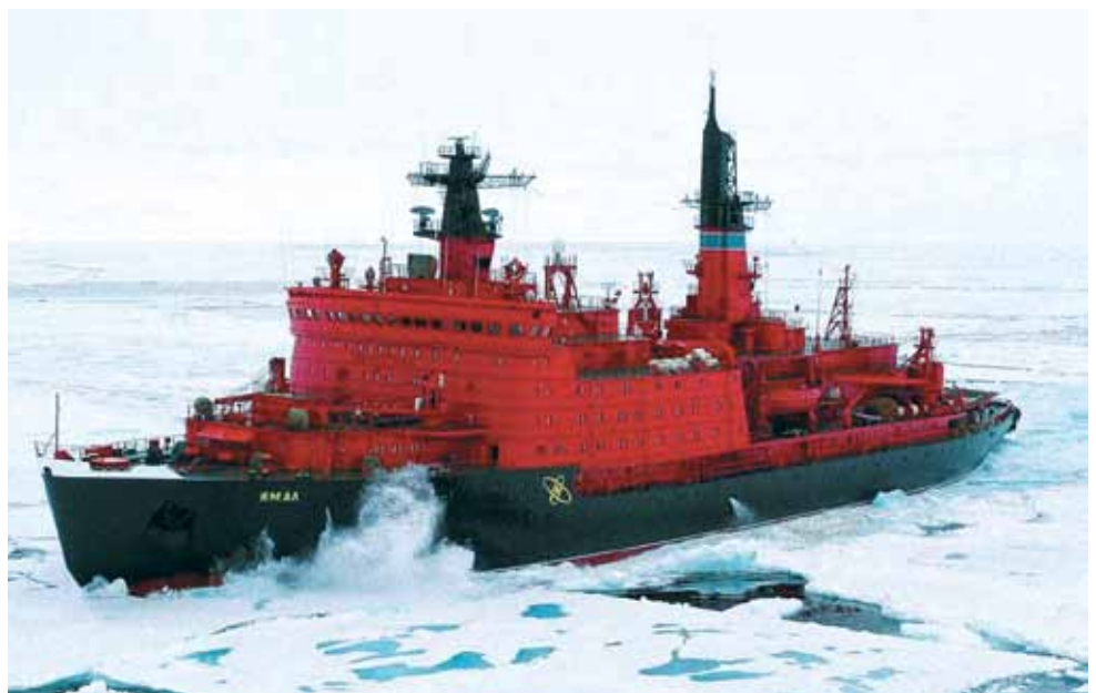
Russia is one of the only countries with a fleet of icebreakers, and they are working on the newest generation of nuclear-powered icebreakers for use in the Arctic. Shown: the Russian nuclear-powered icebreaker Yamal.
