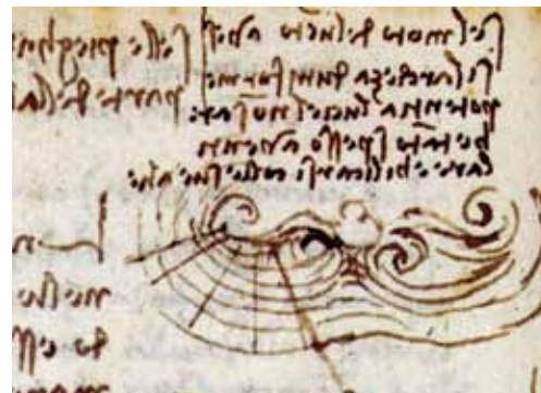
Leonardo's drawing of vortex formation around the bird's wing is from Manuscript E 47 verso. The curvature of the wing, especially at the tips, is directly connected to the curvature of the air underneath it. The straight lines drawn across the airflow represent the centripetal force that presses the wing to curve. (Domenico Laurenza, "Leonardo on Flight," 2004).
