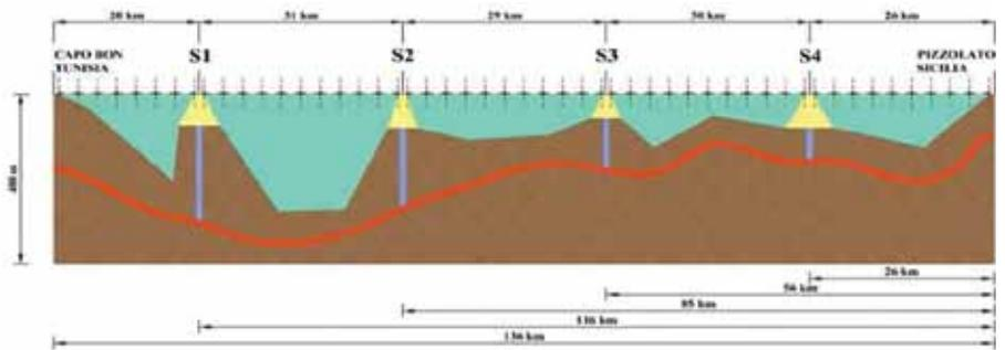
*To cover the entire length of crossing is necessary to create artificial islands, which divide the path into 4 parts; these islands will be the support for the suspended structure of the bridges dividing the path in segments of about 20-30 km each.*
