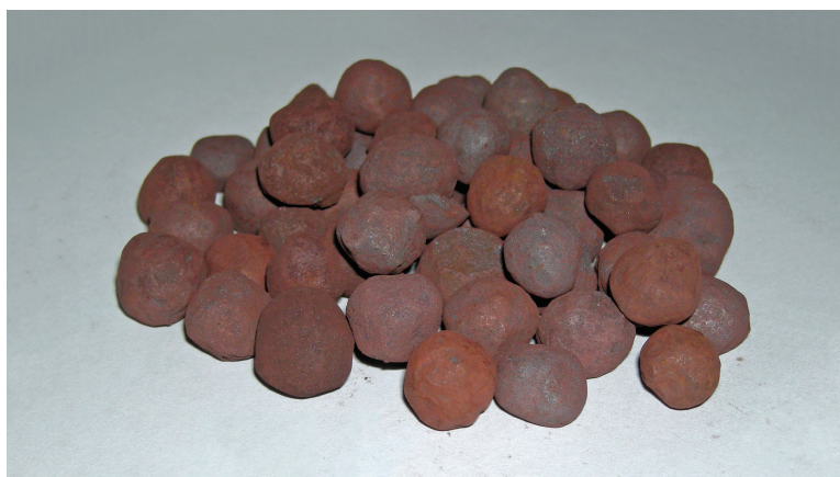
Taconite, a processed form of iron ore, looks like rust. Smelting taconite to produce iron is essentially “un-rusting” it.
