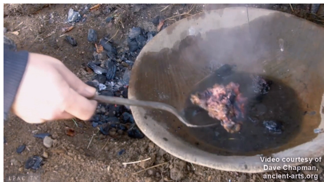
Retrieving copper created from malachite which has been “burned” in a charcoal fire.
