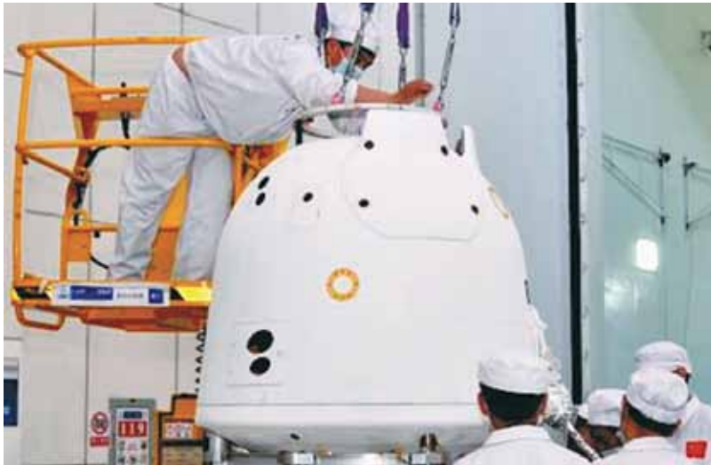
Chang'e 5-T1's re-entry module after vacuum thermal tests.
