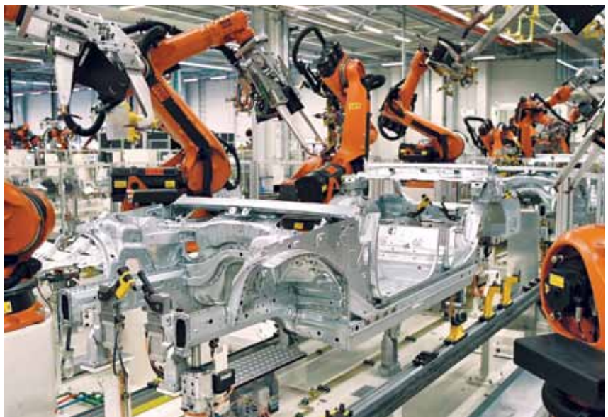
Computer-controlled spot welding in a BMW plant in Leipzig, Germany, using industrial robots manufactured in Germany by KUKA (Keller und Knappich Augsburg).
