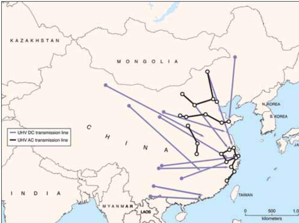
China's UHV electrical transmission lines. The longer blue lines are direct current (DC) with only a single destination, while the shorter black lines are alternating current (AC), which lose more energy but are capable of dispensing energy to several locations.
