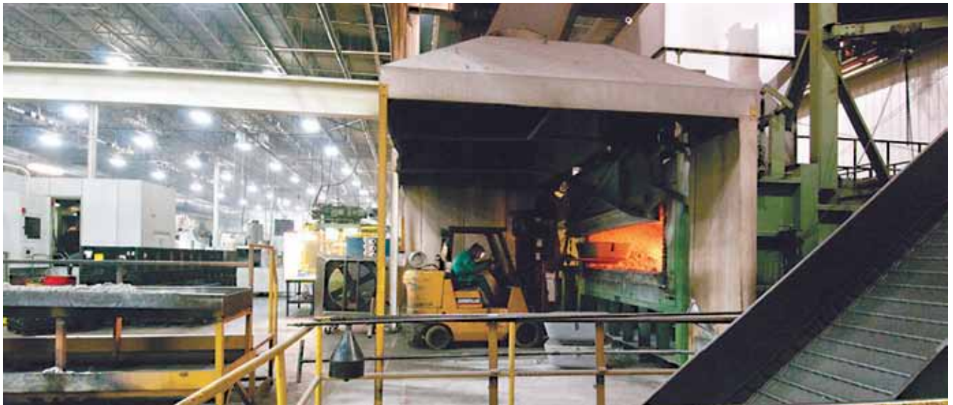
Another view of the Port City Castings facility showing an operator forklifting foundry ingots into the furnace crucible.
