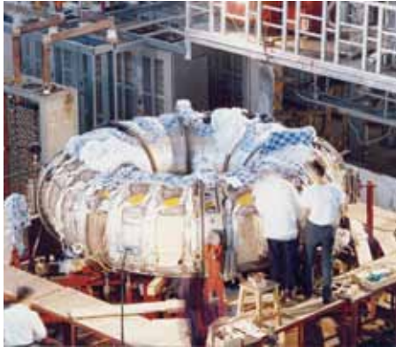
Institute of Plasma Physics, Chinese Academy of Sciences After receiving the discarded T-7 tokamak from the Soviet Union, engineers at the Hefei Plasma Physics Institute disassembled the machine (above) and rebuilt it as HT-7 (right).
