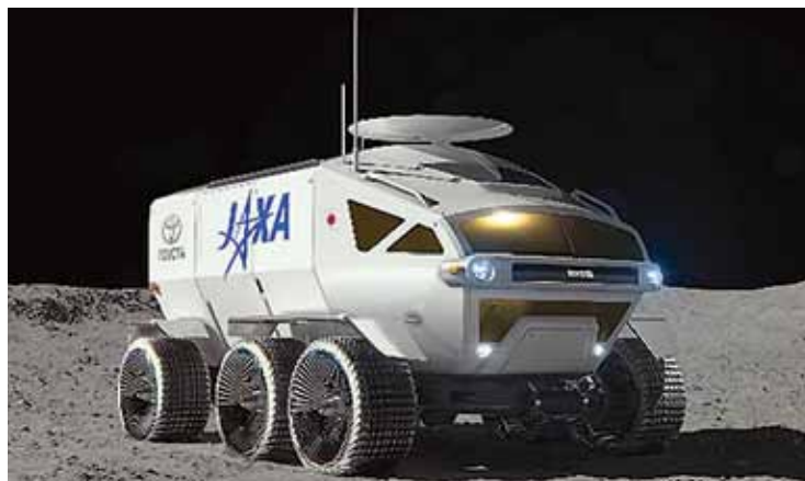
Concept from a joint Japan Aerospace Exploration Agency (JAXA)-Toyota study for a lunar vehicle carrying two astronauts. JAXA is one of many agencies and companies interested in working in the Artemis program.
