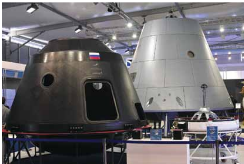
A mockup and test vehicle of Roscosmos' Orel deep space crew module on display at the Moscow Air and Space Show in August 2015.
