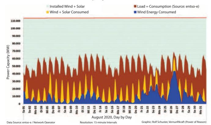
The red line at the top is the amount of solar and wind energy we have installed in Germany. It's far more than we actually need. The peak demand is about 85 GW or 85,000 MW in Germany.
