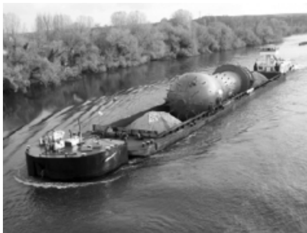
A vessel for a nuclear power plant is towed on a barge along a French waterway. An upgraded Rhine-Rhône canal corridor could become a vast assembly line for floating nuclear power plants.
